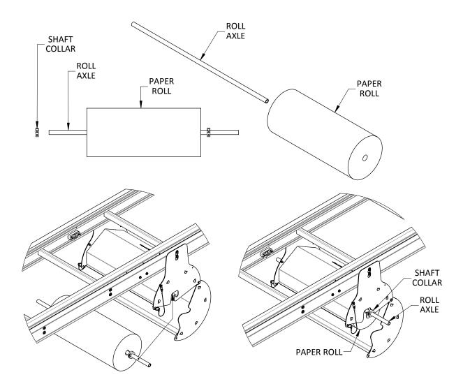
Installing Kraft Paper Roll, Roll Hanger with Enclosure
