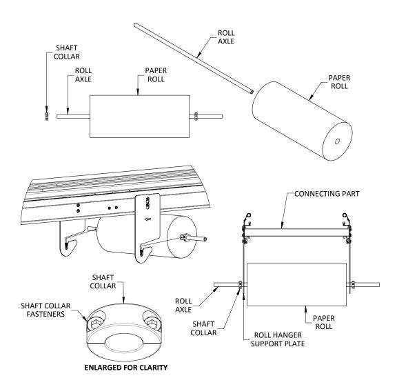
1. Feed Roll Axle through Paper Roll and install Shaft Collars.
