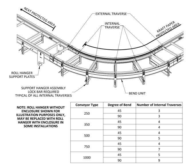
2. If a Bend Unit is encountered, install Support Bar Assemblies and Lock Bar at each internal traverse on Bend Unit.
